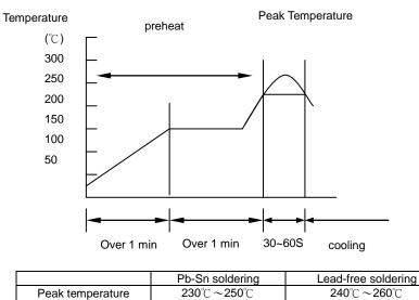
While in preheating, please keep the temperature difference between soldering temperature and surface temperature of chips as: T≤150°C.
