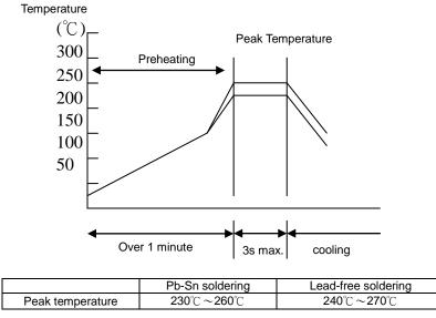
While in preheating, please keep the temperature difference between soldering temperature and surface temperature of chips as: T≤150°C.
